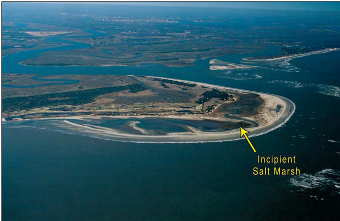
FIGURE 2.7. The eastern end of Kiawah Island in December 1998 [UPPER] and February 2005 [LOWER]. Note the 1989 shoreline situated well inland from the outer beach. Shoals 1 and 2 added upward of 5 million cubic yards to Kiawah in the 1990s. As waves pushed the new sand shoreward, an incipient barrier island/lagoon/marsh formed. The new lagoon was flushed via a channel at the western end of the accreted beach. [From CSE 2007]
