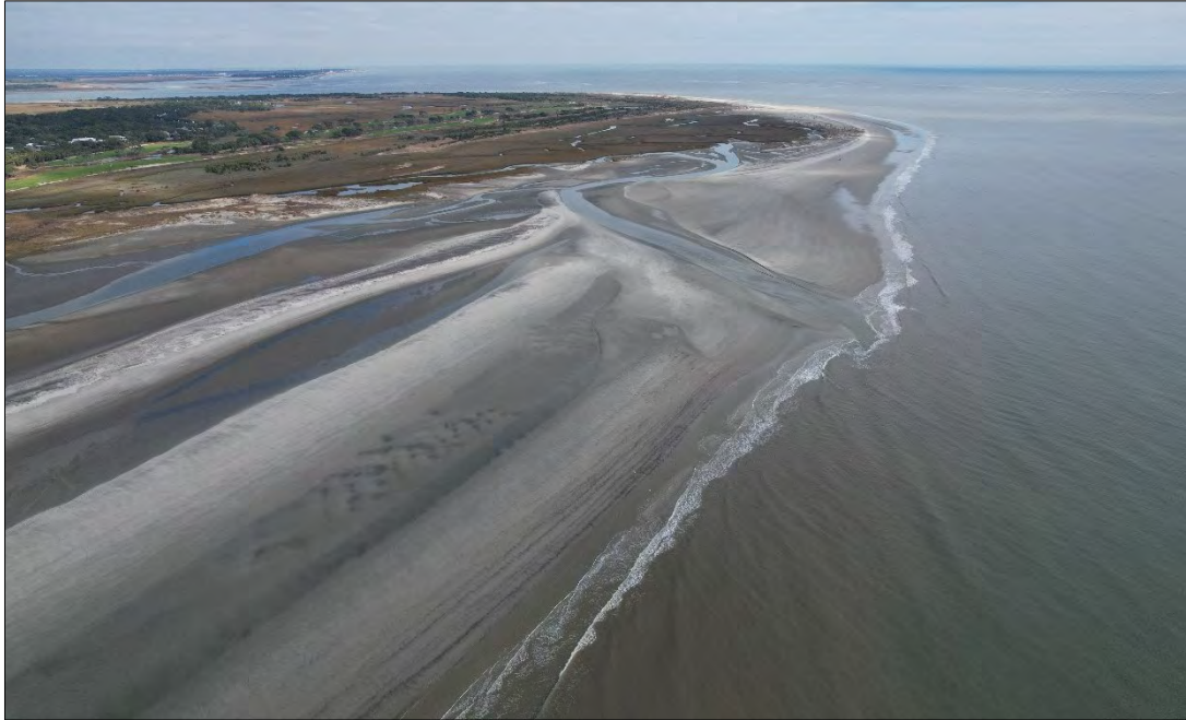
FIGURE 2.2. The East End of Kiawah Island in December 2025. A large shoal has delivered ~1.5 million cy of sand to the East End since ~2019. Measured volume increases as far west as the Beach Club reflect the downcoast spreading of this sand over the last several years.
