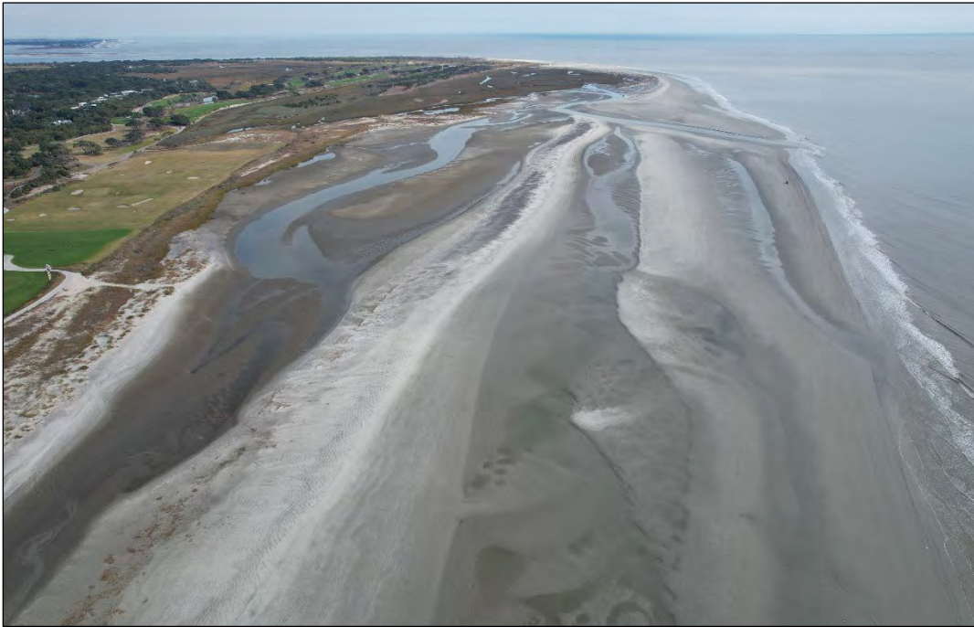
FIGURE 4.7. [UPPER] December 2024 aerial photo over the East End marshes showing the shoal is attaching and feeding sand to the beach between the East End and Stono Inlet (center background). [LOWER] December 2025 aerial photo showing the shoal attached and growing the dry sand portion of the beach.
